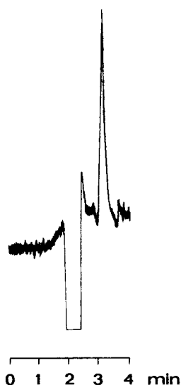
Fig. 2. High-performance liquid chromatogram of a surface water sample from a lake spiked with 4-aminophenol at a concentration of 10 \mu\text{g/l} (10 ppb). Column: LiChrosorb RP-8, 5 \mu\text{m} ( 125 \times 4.6 \text{ mm} I.D.). Mobile phase: 30 ml PIC-A reagent in 1 l water-methanol (80:20); flow-rate, 1 ml/min. Fluorescence detection: excitation, 323 nm; emission, 373 nm.
